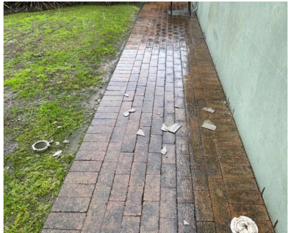
Line ID 2: External, Geriatric Unit Ground Level, South Western Side, Floor, Fibre Cement Sheet Debris - No Asbestos Detected
